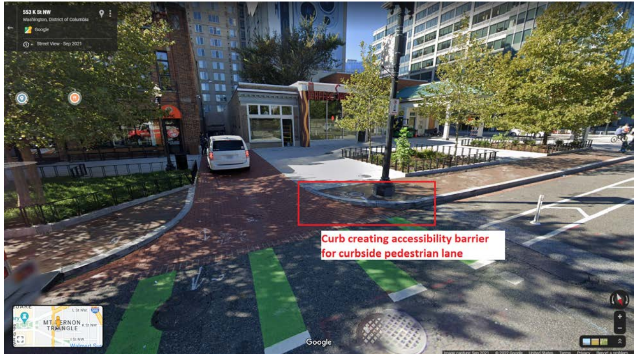
Figure 1: Google Streetview at the location of the proposed unenclosed sidewalk cafe. Note the curb stepping down from the bricked portion of the sidewalk to the public alley, which creates an accessibility barrier.
